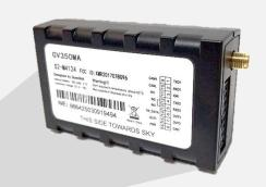
Network Operating Band for North America: LTE eMTC/NB-IoT LTE B2/B4/B5/B12/B13
